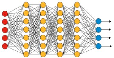
Example of an artificial neural network with four hidden layers in yellow, one input layer in red and one output layer in blue.
